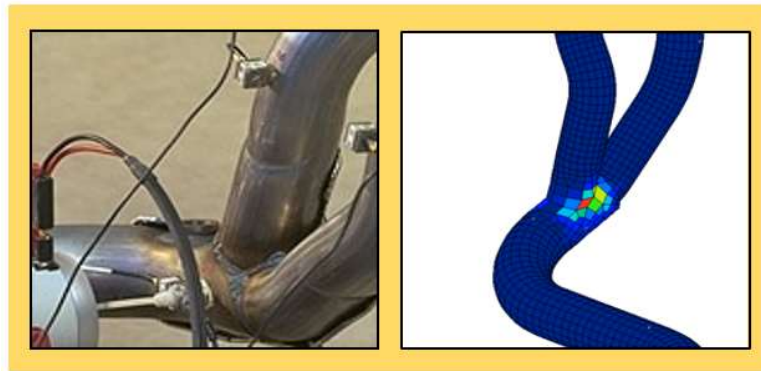
Figure 10: Welds at the Y pipe joint of the physical exhaust system (left) had to be introduced into the finite element model (right) to achieve better correlation.
