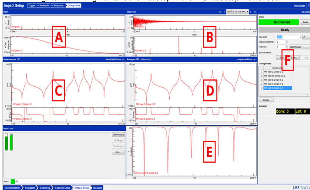
Figure 16: Driving Points is the last step in the Impact Setup worksheet.
