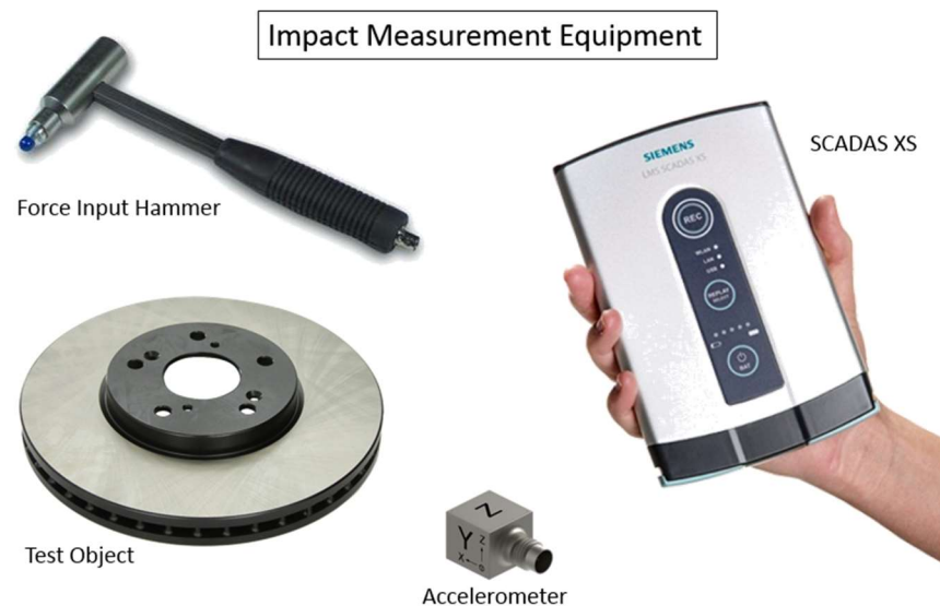
Figure 1: Impact measurement equipment
