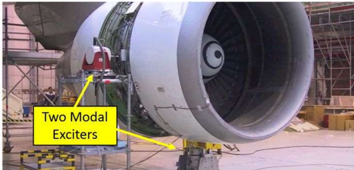
Figure 7: A structural test on aircraft engine with two modal shaker exciters. During the test, these exciters will probably exhibit coupling.
