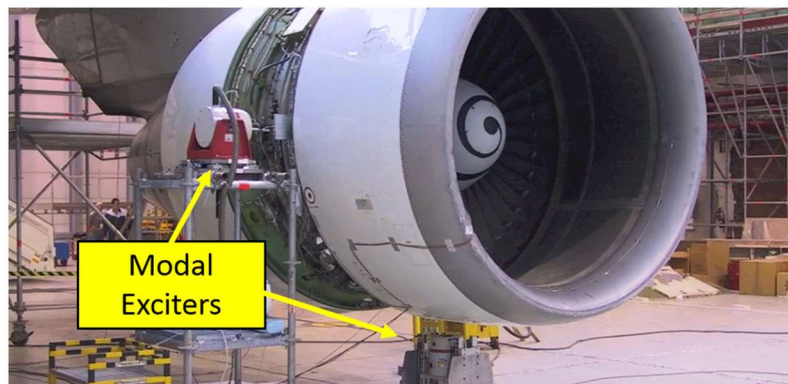
Figure 5: Lateral exciter (on left side) and vertical exciter (on bottom) for an aircraft engine.
