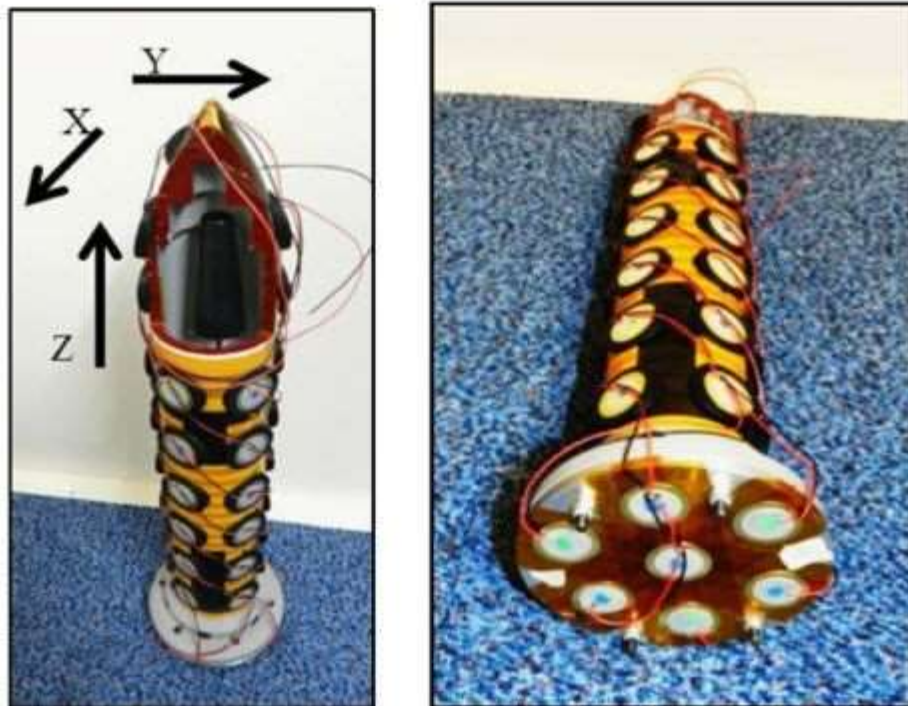
Figure 6: Multiple Exciters applying excitation energy in several different axes at many points on the structure allow a better distribution of energy to achieve better results in terms of responses around the structure. This case was to simulate the excitation forces due to aerodynamic loading.
